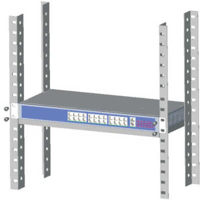
Figure 2-2 Install switch to the rack
